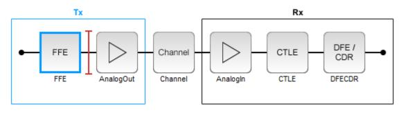
Select the FFE block in the Tx subsystem. In the Block Parameters window, change **Tap weights** from  $[0 \ 1 \ 0 \ 0]$  to  $[0 \ 1 \ 0 \ 0]$ , so that the FFE has one pre tap, one main tap, and two post taps. Leave all other blocks in their default settings.
